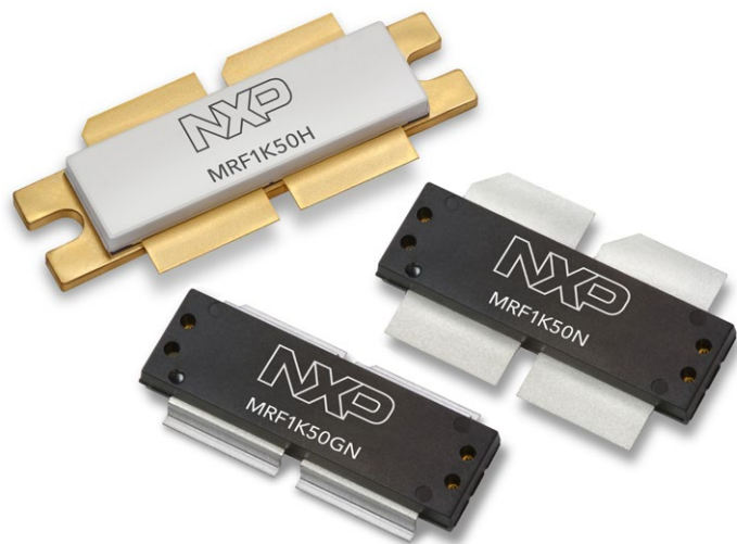
Figure 1: NXP's new LDMOS 1.5 kW RF power transistors, shown here in their three packaging variants, produce the highest CW RF output power of any semiconductor device. The air-cavity ceramic version is pin-compatible with existing transistors – only light retuning is needed to obtain the highest power.
